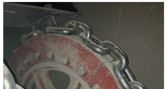
An example of a bucket elevator with gravity discharge, chain ends with chain shackles and force-locking drive
