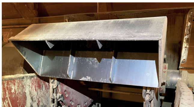
An example of a bucket elevator with centrifugal discharge, conveyor chains and positive-locking drive.
