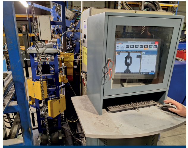
2. Chain calibration, tensile testing, continuous quality control
