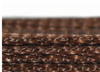
Webbing sling 4-layer structure
