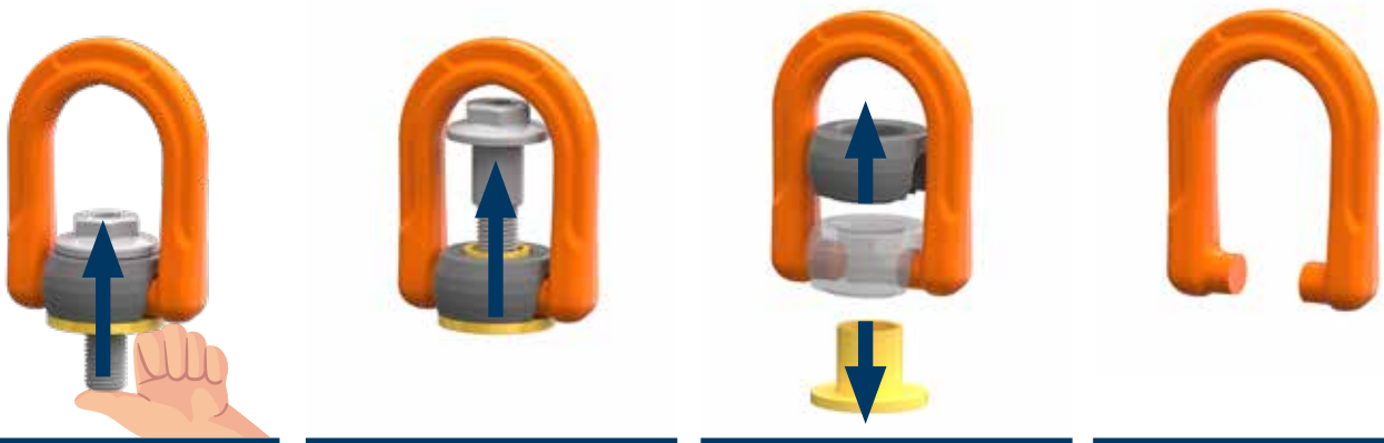
Figure 3: Disassembly of the PLZW (also possible with a tool for the PLZW-FIX-SP)
