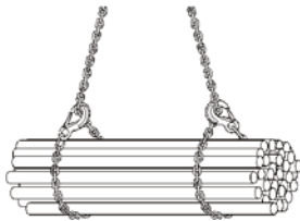
Figure 12: Reverse choke hitch
