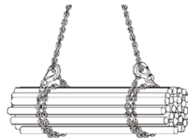
Figure 13: Reverse wrap and choke hitch
