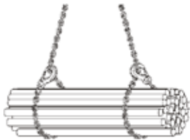
Figure 12: Reverse choke hitch
