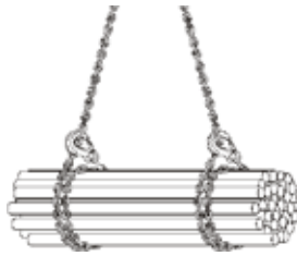
Figure 11: Wrap and choke hitch in the same direction
