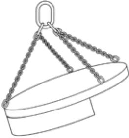
Figure 14: All the load is carried by one chain leg
