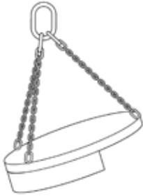
Figure 15: All the load is carried by two chain legs
