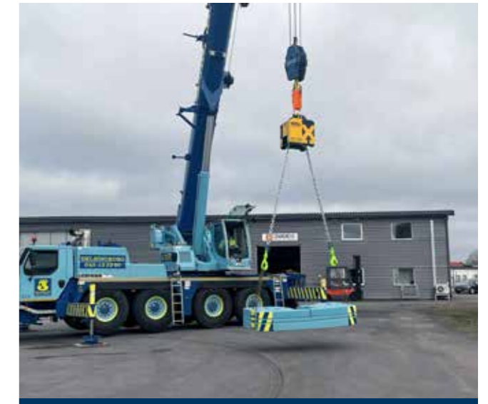
Levo load balancer equalising crane counter weight
