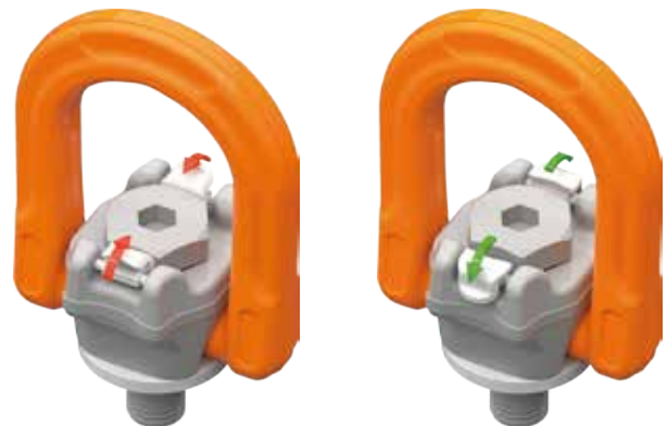
Picture 4: Position 'A' – both latches are touching the screw. Only permitted during mounting and demounting.
