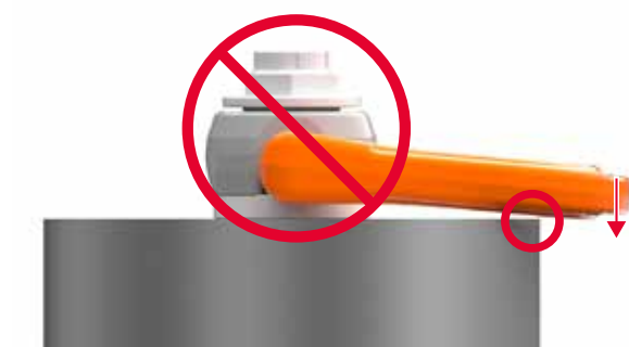
Improper loading as loading ring rests against edges or surfaces
