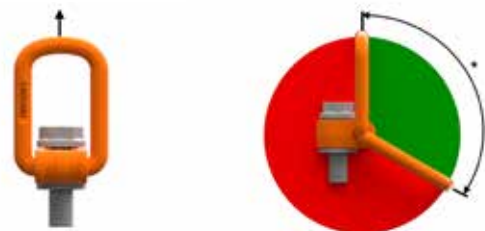
Pic. 1: Permitted directions of load that occur during correct use. * Ring may not touch the load
